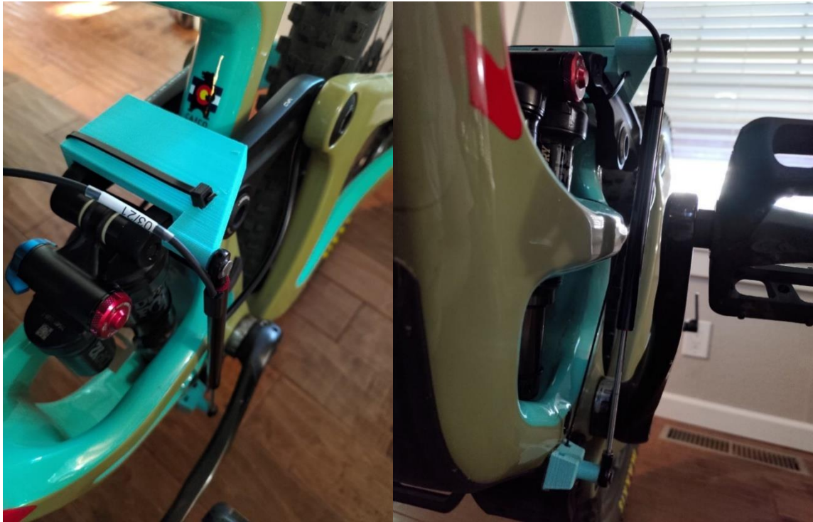
Figure 16: Linear Potentiometer System on Bike
